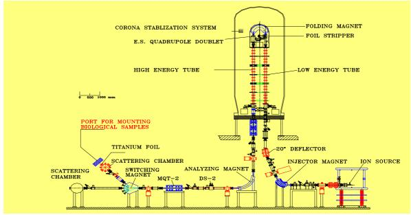
Fig. 2: Schematic diagram of the 6 MV Folded Tandem Ion Accelerator
