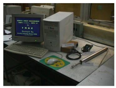
The software, which was developed in C language, was modified such that it takes care of different types of temperature correction factors to be applied on measured creep value for different combinations of pressure tube material and geometrical layout. It was also made compatible to ADC-528.
